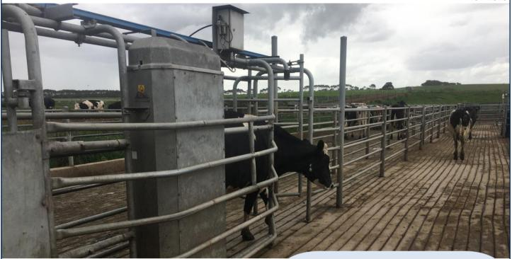
Auto-drafting is an electronically-operated gate that automatically sorts cows via their Electronic Identification.
