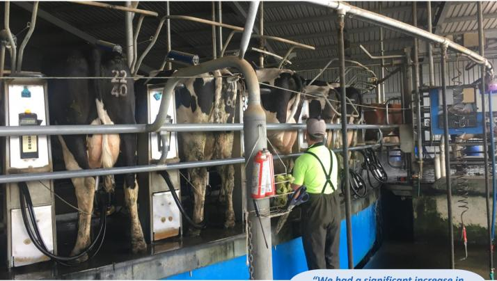
In-line milk meters generate data on milk production and the milking process for every cow at every milking. All meters measure milk yield. Some test biological indicators for mastitis, nutritional or reproductive status.
